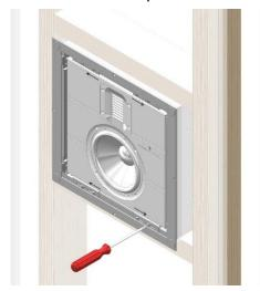
Mount the grill by pushing it gently onto the frame until it snaps into place.
