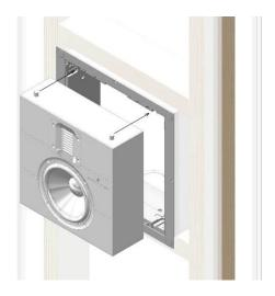
Slide the brackets back into place for securing the speaker. Tighten the screws.
